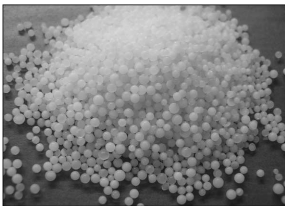
Fig. 4 Silica supported TFESA (@1.5 mm beads).
